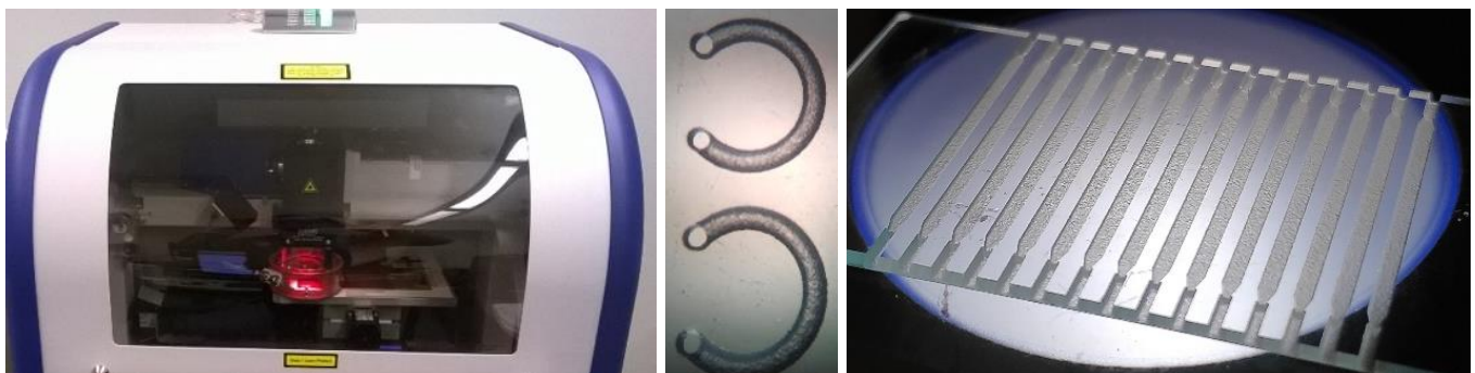
Laser micromachining device (left) used to fabricate C-shaped (middle), and straight (right) microchannels.
