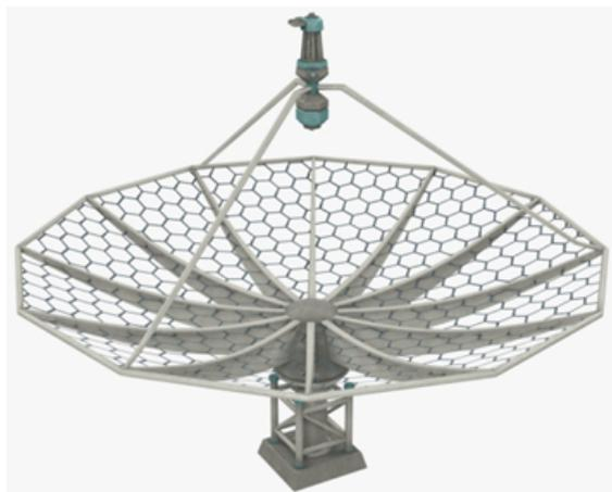
Figure 5-10 Flexible array overlaid on parabolic frame to produce enhanced dish antenna.
