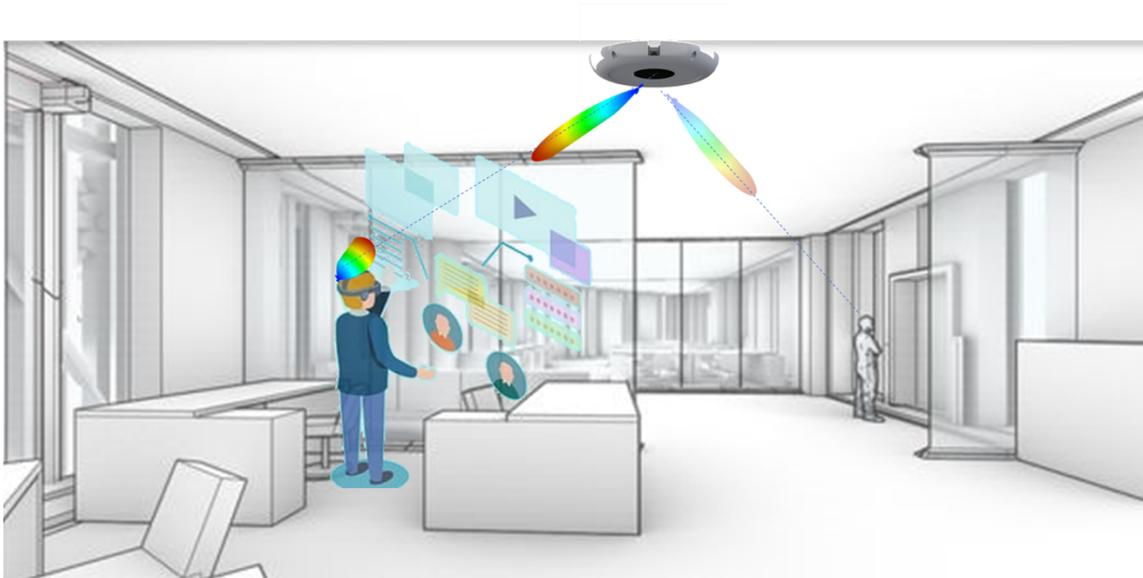
Figure 6-19 Indoor direct short-range link for immersive data analysis and exchange
